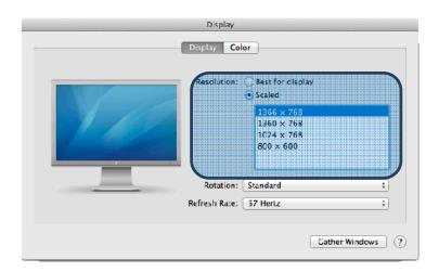
The resolutions available depend on both the DisplayLink enabled product and the capabilities of the connected display.
